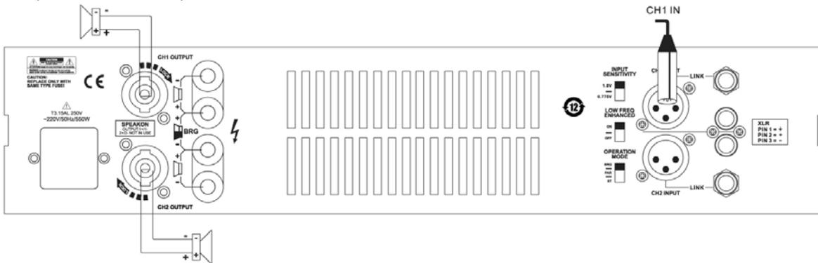
In this mode, connect the CH1 input to the sound source (such as mixer, CD) output, set the mode at "PARALLEL", adjust the two channels volume to a suitable position, connect the two SPEAKON to two speakers.
