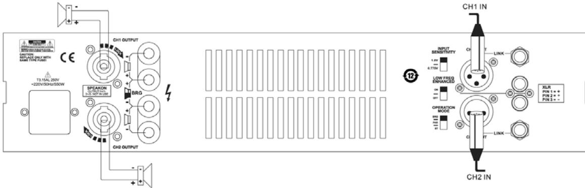
In this mode, connect the two channels input to the sound source (such as mixer, CD) output, set the mode at "STEREO", adjust the two channels volume to a suitable position, connect the two SPEAKON to two speakers.
