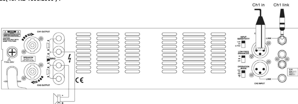
In this mode, connect the CH1 input to the sound source (such as mixer, CD) output, set the mode at "BRIDGE" adjust the CH1 volume to a suitable position, connect the BRIDGE OUTPUT to the speaker.
