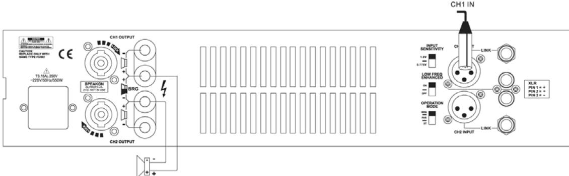
In this mode, connect the CH1 input to the sound source (such as mixer, CD) output, set the mode at "BRIDGE" adjust the CH1 volume to a suitable position, connect the BRIDGE OUTPUT to the speaker.
