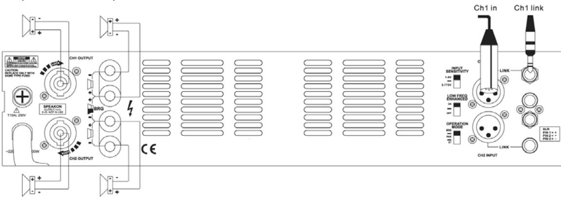
In this mode, connect the CH1 input to the sound source (such as mixer, CD) output, set the mode at "PARALLEL", adjust the two channels volume to a suitable position, connect the two SPEAKON to two speakers.
