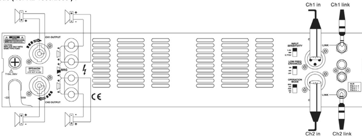
In this mode, connect the two channels input to the sound source (such as mixer, CD) output, set the mode at "STEREO", adjust the two channels volume to a suitable position, connect the two SPEAKON to two speakers.
